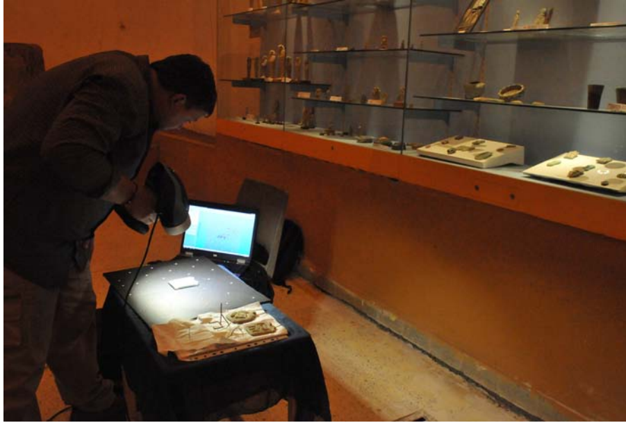
Fig. 7 – Scanning of small objects (Object No. 6.1) placed on a plate with pre-attached positioning targets by VIUscan. Photo Jaroslav Kroužek.
