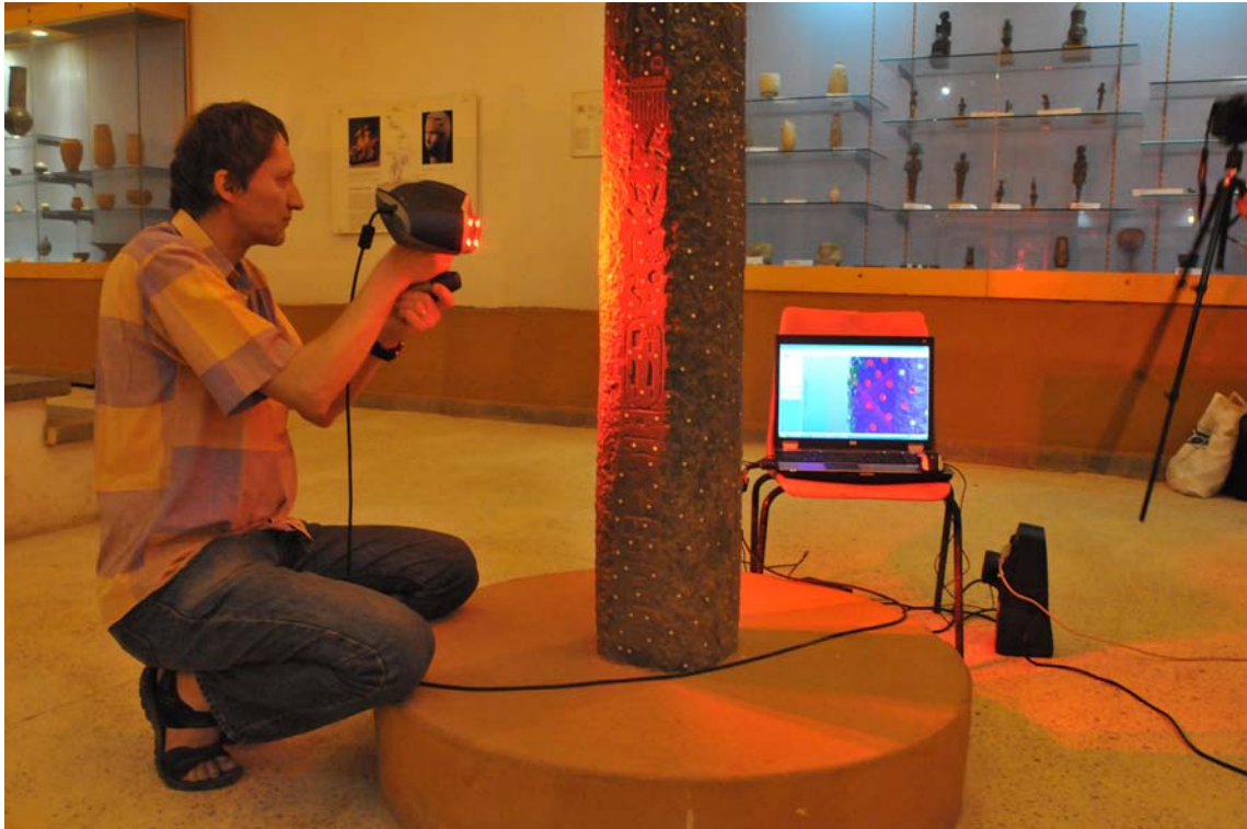
Fig. 3 – Scanning with the EXAscan 3D handy scanner. Photo Jaroslav Kroužek.
